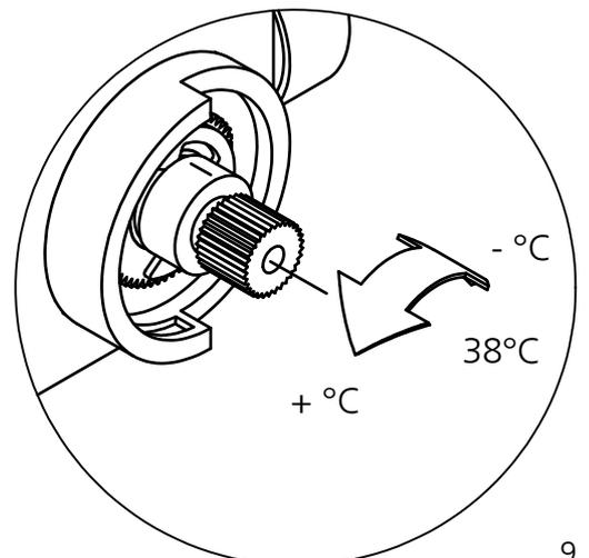
BYTE AV TERMOSTAT/CARTRIDGE EXCHANGE
